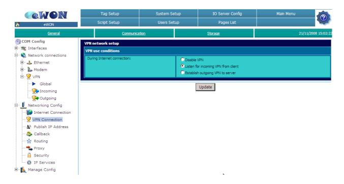
Make sure that the VPN network setup is on «Listen for incoming VPN from client».
