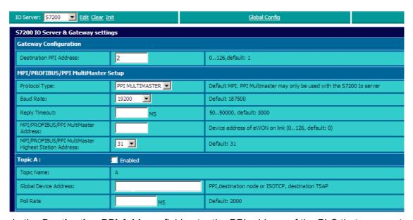
In the **Destination PPI Address** field enter the PPI address of the PLC that you want to access remotely. In **Protocol Type**, select **PPI Multimaster**.
