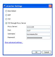
Select connection *TCP through proxy server* and encode your Proxy settings inside the Proxy server box. To save the settings, click on *OK*.
