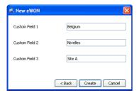
Here you can enter additional information concerning your remote connection. The *Custom Fields* can be used to classify or filter your different remote connections. This will allow you to find easily the eWON you need to connect to.
