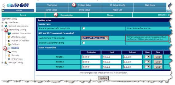
**Note**: For earlier eWON firmware versions, the eWON LAN IP address has to be manually specified as gateway on the connected device (see our device manufacturer specific user guides).
