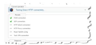
The Talk2M registration will now start and the result will be displayed on the wizard page: The eWON will first test the different connections needed to connect to the Talk2M server (UDP and HTTP or HTTP using a Proxy).
