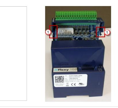
Hooks to be pressed are off-centered – press while pulling upwards
