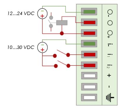
The digital output is activated by an open drain MOSFET transistor driven by an optocoupler. The maximum current flow inside this transistor has a value above the one specified in the eWON, in order to cope with the switching power losses.
