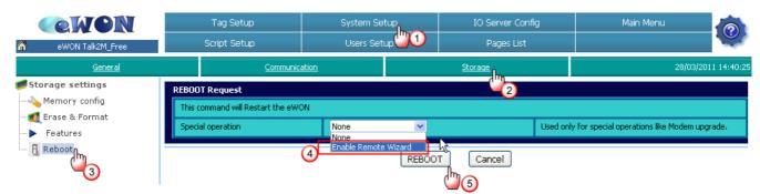
Select the **Enable Remote Wizard** option in the **Special Operation** field and click on the **REBOOT** button. The eWON will reboot and launch the remotewizard.txt file.
