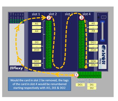
**Note**: Following the left-to-right order of slots, the first card to be detected is the Extension Card plugged in the most left slot, then the next on its right and so on. Removing an I/O card other than the utmost right one will result in an internal reallocation of tag addresses. To avoid a mismatch between physical I/Os and their software configuration, the software
