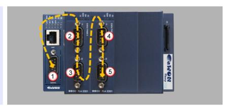
The detected cards (5) appear in the eWON System hardware configuration page like shown here (slots 1 & 2).
