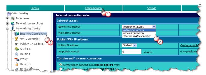
Choose for example the "Ethernet WAN connection", to use the second Ethernet card (Ethernet WAN) of the eWON for the Internet connection.
