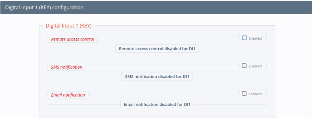
To enable the the remote access control, simply click the enabled check box.
