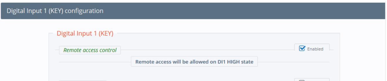
If enabled, the remote access through Talk2M will only be possible if the state of the digital input 1 is high, so only if the Key Switch has been enabled.
